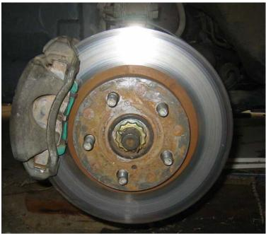
These started out as my original front brakes, & because I'm more of a twisty road person, than straight line speed, I didn't think they'd be adequate. These are a single piston floating calliper.
