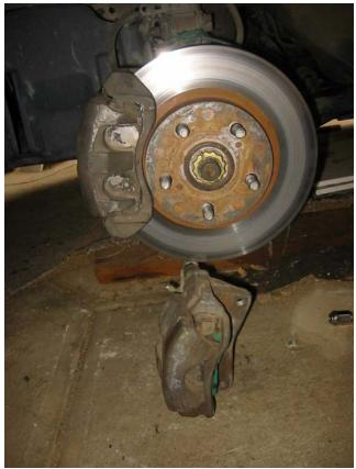
The only mod needed was to grind away some of the brake backing plate to clear the calliper.
