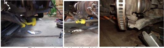
This was solved with a bit of "clearance grinding".
